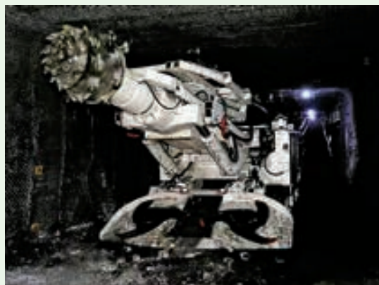
Integrated Excavator Applied for Spraying
